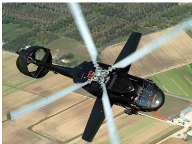
图2 “速度鹰”(Speed Hawk)和其“环形尾” Fig.2 Speed Hawk and its ducted propeller
