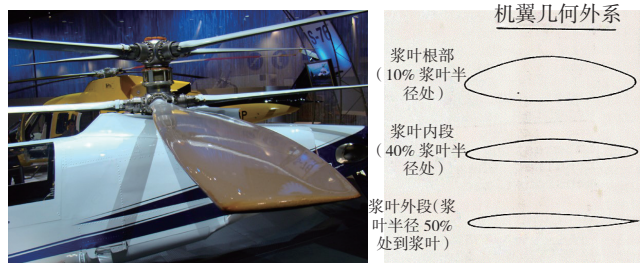
图15 西科斯基X2的翼型分布和桨叶实体外形 Fig.15 Sikorsky X2 airfoil distribution and blade profile
